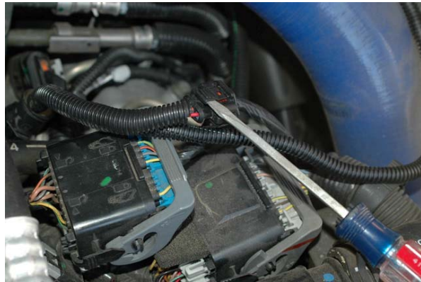
Screwdriver orientation shown to speed insertion and removal of connector
